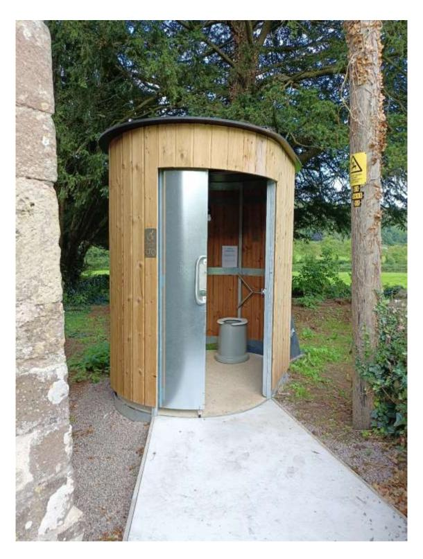
This is a really clever system that uses the effect of the sun and wind to drive significant evaporation, meaning that very little remains once the work of the wind and sun has been done. The system also makes use of the breeze being drawn down through the bowl of the loo, which means there is no smell and the cabin is made from aromatic cedar wood.
